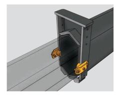
**Side supports for stability** *Side supports fitted on each boom extension stabilize the boom laterally and minimize the play. Most Hiab crane models can be delivered with extension*
